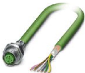
Bus system flush-type socket, INTERBUS, 5-pos., M12, shielded, B-coded, rear/screw mounting with M16 thread, with 1 m bus cable, 3 x 2 x 0.25 mm 2
