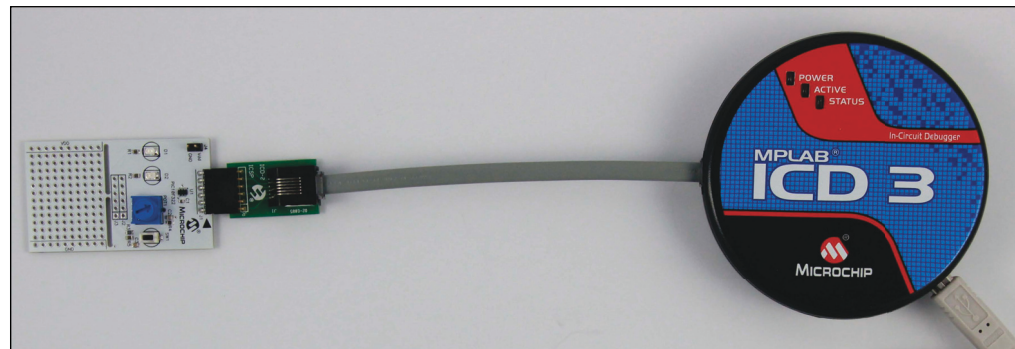
FIGURE 1-3: CONNECTING THE MPLAB® ICD 3 TO THE PIC10(L)F32X DEVELOPMENT BOARD
