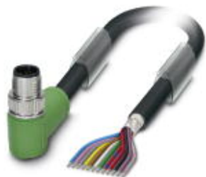
Sensor/Actuator cable, 12-position, PUR/PVC, Black RAL 9005, shielded, Plug angled M12 SPEEDCON, A-coded, on free cable end, Cable length: 10 m
