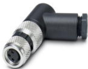
Connector, 3-position, Socket angled M8, A-coded, Screw connection, Knurl material: Nickel-plated brass, External cable diameter 3.5 mm ... 5 mm
