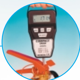
CFG Testing fire extinguisher
