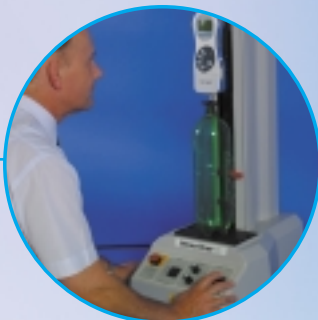
Top load bottle test
