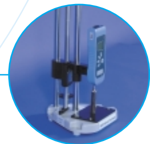
BFG on MDD manual test stand
