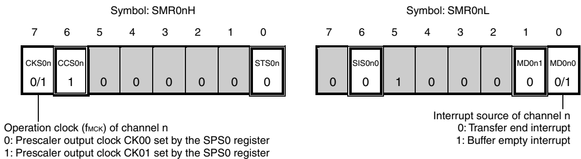
Figure 10-62. Example of Contents of Registers for Slave Transmission/Reception of 3-Wire Serial I/O (CSI00) (1/2)
