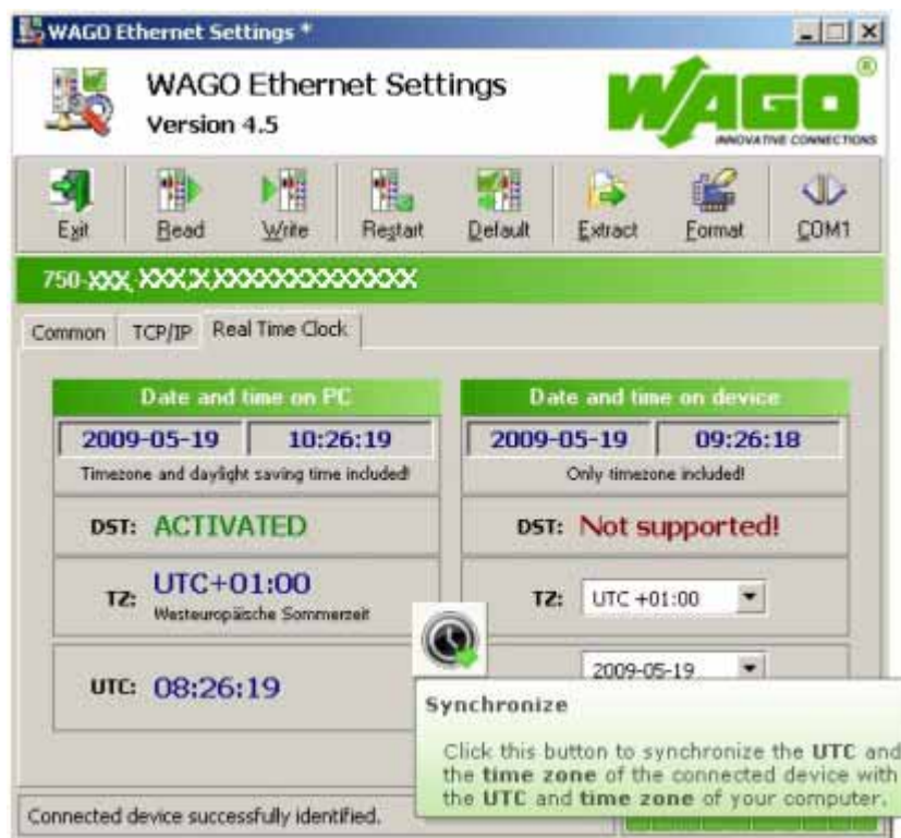
Figure 54: Example of real-time clock synchronization in ETHERNET Settings
