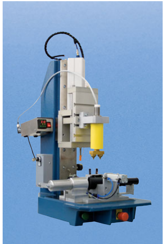
KVT Basic 2500 thermal installation machine for simultaneous thermal installation of two inserts into a car charge air pipe
