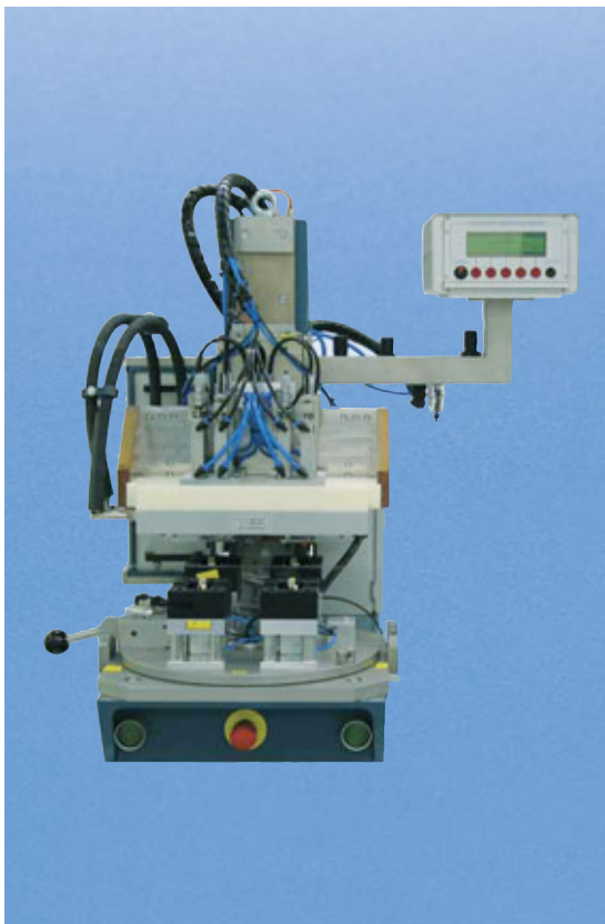
ERW thermal installation machine to embed eight inserts M 1.6 into two mobile phone half shells
