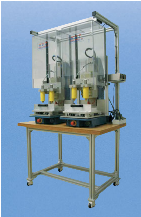
KVT Basic 5000 DUO thermal installation machine for simultaneous thermal installation of four inserts into two covers of car outside mirrors
