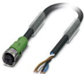
Sensor/Actuator cable, 4-position, PUR, black-gray RAL 7021, free cable end, on Socket straight M12 SPEEDCON, A-coded, Cable length: 2 m
