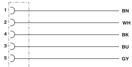
Contact assignment of the M12 socket
