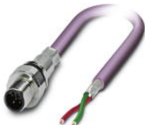
Bus system flush-type plug, PROFIBUS, 2-pos., M12, shielded, B-coded, front/screw mounting with M16 thread, with 10 m bus cable, 2 x 0.25 mm 2
