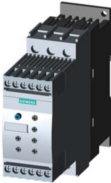
SIRIUS SOFT STARTER, S0, 12.5A, 5.5KW/400V, 40 DEGR., AC 200-480V, AC/DC 110-230V, SCREW TERMINALS
