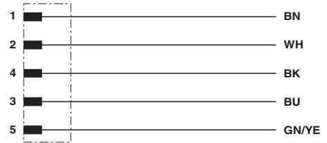
Contact assignment of the M12 plug
