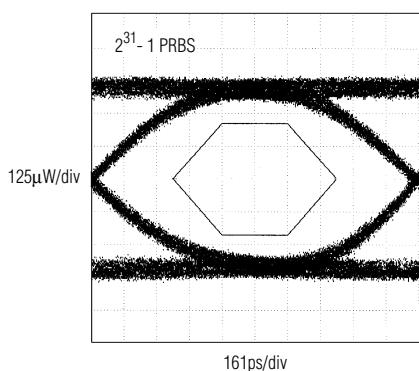
EYE DIAGRAM (622Mbps, 1300nm LASER, 470MHz FILTER)
