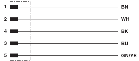
Contact assignment of the M12 plug
