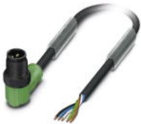
Sensor/Actuator cable, 5-position, PUR halogen-free, black-gray RAL 7021, Plug angled M12, A-coded, on free cable end, Cable length: 3 m, with plastic knurl
