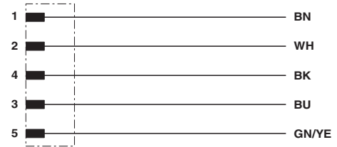
Contact assignment of the M12 plug
