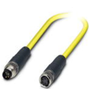
Sensor/Actuator cable, 4-position, PVC, yellow, shielded, Plug straight M8, on Socket straight M8, Cable length: 1.5 m
