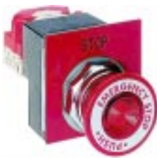
For “emergency-stop” applications, a standard Type KA contact block is mounted to the push button module. The Type KA block provides a direct acting hard contact break required by code for “e-stop” applications, while the SERIPLEX module provides a quick indication (to the host) of the “e-stop” signal location. This application is good for long conveyors and other industrial uses where numerous “e-stop” locations are required.
