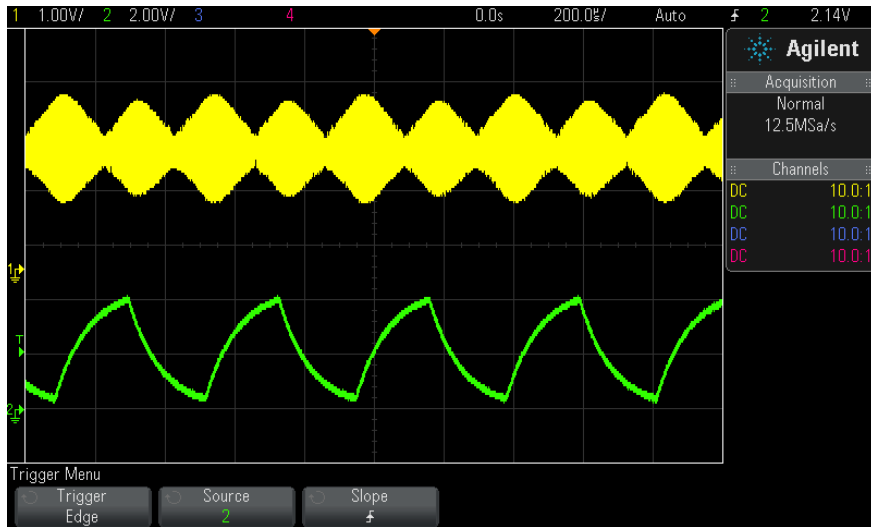
Figure 13 Amplitude Modulation Shown at 100% Intensity
