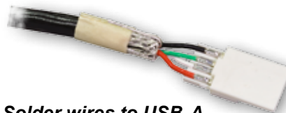
Solder wires to USB-A Insert
