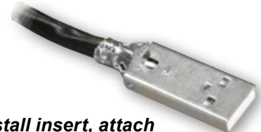
Install insert, attach lid, and crimp shield
