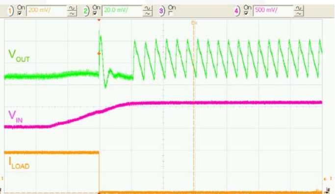
Figure 23. Combined Line/Load Transient 3.3 to 3.9V_{IN} Combined with 400mA to 40mA Load Transient
