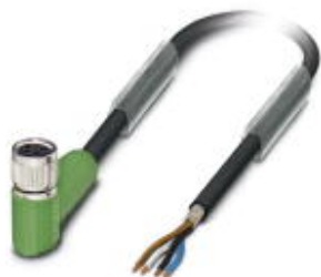
Sensor/Actuator cable, 4-position, PUR halogen-free, black-gray RAL 7021, shielded, free cable end, on Socket angled M8, Cable length: 10 m
