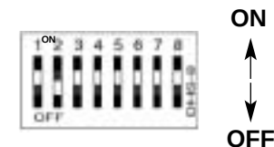
Figure 4. Close up of configuration switches
