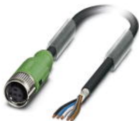
Sensor/Actuator cable, 5-position, PUR halogen-free, black-gray RAL 7021, shielded, free cable end, on Socket straight M12 SPEEDCON, A-coded, Cable length: 10 m
