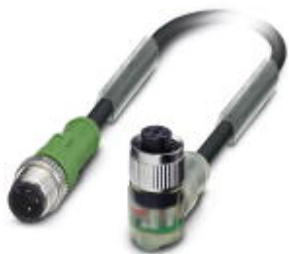
Sensor/Actuator cable, 3-position, PUR halogen-free, black-gray RAL 7021, Plug straight M12, A-coded, on Socket angled M12, A-coded, with 2 LEDs, PIN 2+4 bridged, Cable length: 0.6 m
