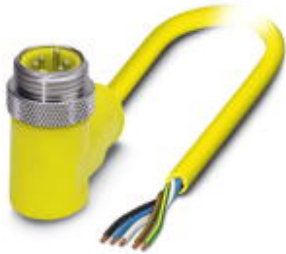
Sensor/Actuator cable, 5-position, PVC, Yellow RAL 1021, Plug angled 7/8"-16UNF, A-coded, on free cable end, Cable length: 6 m
