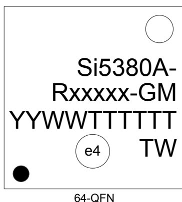
Figure 12.1. Si5380 Top Marking
