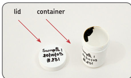
Mark both lid and container to avoid mismatch (Grease quantity in the picture is 0.5 gram, 0.02 oz)
