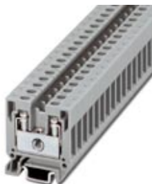
Mini feed-through terminal block, Connection method: Screw connection, Cross section: 0.2 mm 2 - 4 mm 2 , AWG: 24 - 12, Width: 6.2 mm, Color: gray, Mounting type: NS 15
