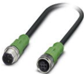
Sensor/Actuator cable, 3-position, PVC, Black RAL 9005, Plug straight M12, A-coded, on Socket straight M12, A-coded, Cable length: 5 m
