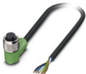
Sensor/Actuator cable, 5-position, PVC, Black RAL 9005, free cable end, on Socket angled M12, A - standard, Cable length: 10 m
