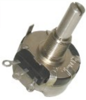
53 Series Industrial Potentiometer, Conductive Plastic Element, Solder lug Terminals, 2 W Power Rating, 50 Ohm Resistance Value
