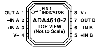
Figure 5. ADA4610-2 Pin Configuration, 8-Lead LFCSP_VD (CP Suffix)
