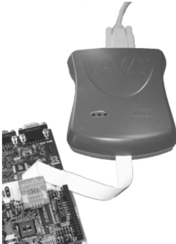
Figure 1-4. Emulating with JTAG ICE
