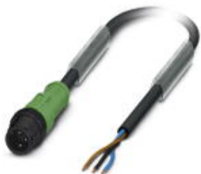
Sensor/Actuator cable, 3-position, PUR halogen-free, black-gray RAL 7021, Plug straight M12, A-coded, on free cable end, Cable length: 5 m, with plastic knurl
