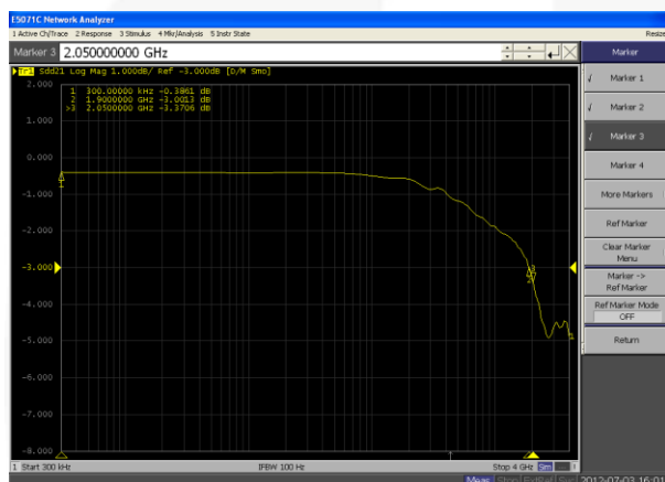
Figure 17. MHL Path SDD21 Insertion Loss Curve
