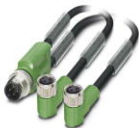
Sensor/Actuator cable, 3-position, PUR halogen-free, black-gray RAL 7021, Plug straight M12, A-coded, on Socket angled M8 and Socket angled M8, A-coded, Cable length: 3 m
