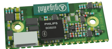
Picture 3: CB-OEMSPA331i-06 OEM Serial Port Adapter long range with internal antenna and a JST 6-pol connector
