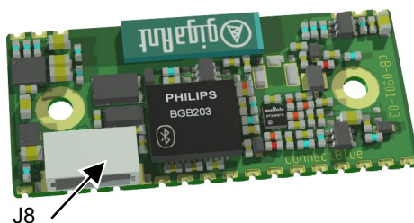
Picture 6: JST 6-pol connector, J8.
