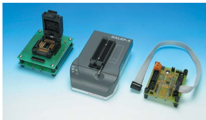
GALEP IV is a professional palm-sized field programmer with universal I/O capability.
