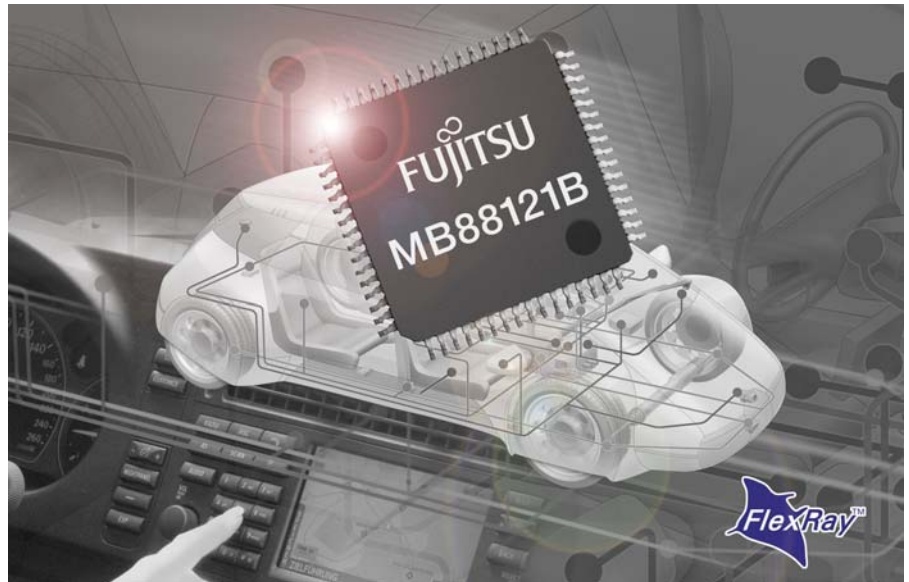
MB88121B adds FlexRay connectivity to 16-bit and 32-bit microcontrollers that lack embedded FlexRay protocol engines.
