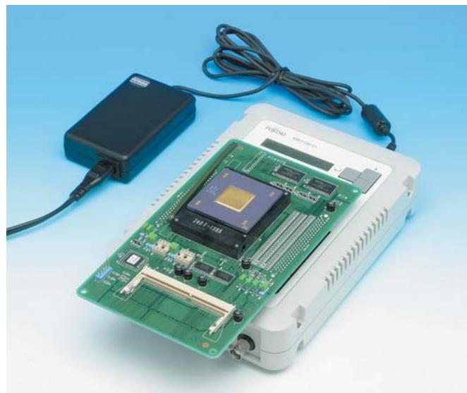
MB2198-01 Fujitsu's emulation system for 32-bit RISC architecture.
