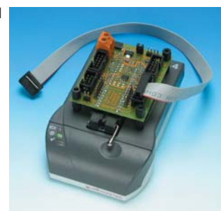
GALEP IV is a professional palm-sized field programmer with universal I/O capability.
