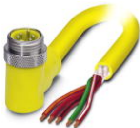
Sensor/Actuator cable, 5-position, PVC, Yellow RAL 1021, Plug angled 7/8"-16UNF, A-coded, on free cable end, Cable length: 2 m
