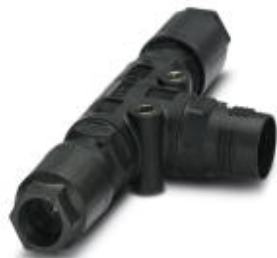
QUICKON T-distributor, black, 4+PE-pos., 1.0 mm 2 ... 2.5 mm 2 /690 V/20 A, for cable diameter of 9 mm ... 16 mm, with two QUICKON nuts
