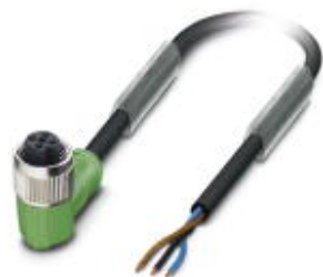
Sensor/Actuator cable, 3-position, PUR halogen-free, black-gray RAL 7021, free cable end, on Socket angled M12, A-coded, PIN 2+4 bridged, Cable length: 5 m
