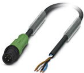
Sensor/Actuator cable, 4-position, PUR halogen-free, black-gray RAL 7021, Plug straight M12, A-coded, on free cable end, Cable length: 5 m, with plastic knurl
