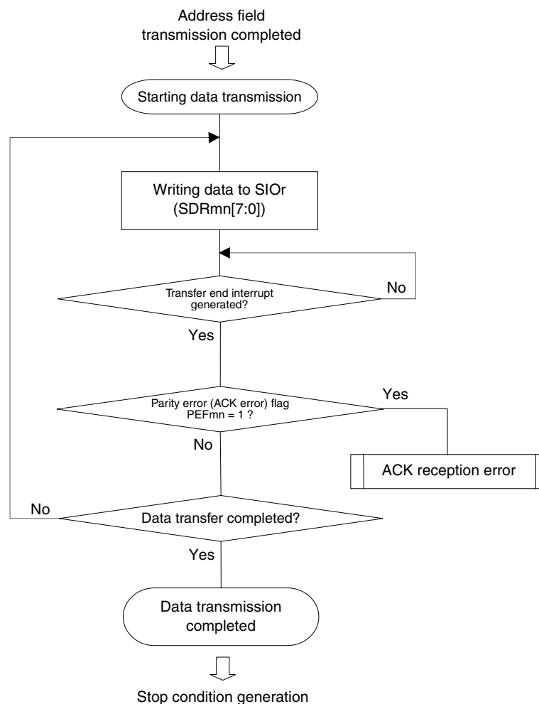
Figure 12-99. Flowchart of Data Transmission
