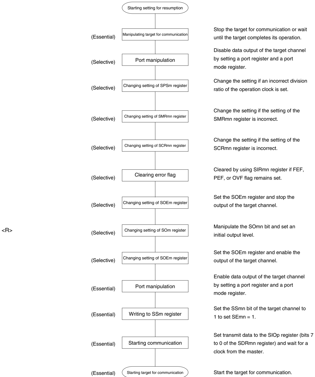
Figure 12-51. Procedure for Resuming Slave Transmission
