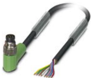
Sensor/Actuator cable, 8-position, PUR halogen-free, Black RAL 9005, Plug angled M8, on free cable end, Cable length: 3 m
