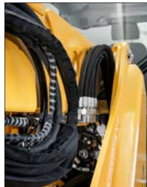
Helagain HEGWS: The ideal protective sleeve for hydraulic hoses.
