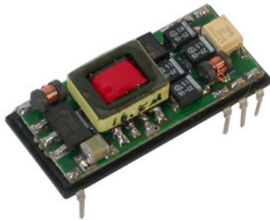
Figure 3: Bobbin-type machine-wound transformer construction in a DC/DC converter. (For a High-Res-Photo, please click on the image!)
