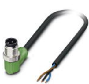
Sensor/Actuator cable, 3-position, PVC, Black RAL 9005, Plug angled M12, A-coded, on Free cable end, Cable length: 2 m
