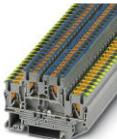
Protective conductor double-level terminal block, connection method: Push-in connection, cross section: 0.14 mm 2 - 4 mm 2 , AWG: 26 - 12, width: 5.2 mm, color: gray, mounting type: NS 35/7,5, NS 35/15
