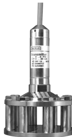
Optional Wika LevelGuard Anti-clog attachment for submersible level transmitters. For use in lift stations, wet wells and other difficult level applications. For more information request bulletin LG-1.
